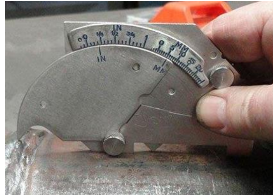
Figure 2 The smallest details are important for the life of the equipment, e.g. weld reinforcement height.
